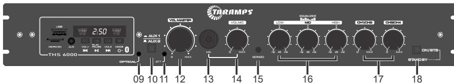
**9 - OPTICAL:** LED indicating the presence of an optical signal. Indicates that the current auxiliary input is optical.
