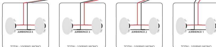
To connect to ceiling speakers, use cables with a minimum gauge of  $1.5\text{mm}^2$  for up to 40 meters. For longer distances, see table on page 02 "Important recommendations". It is necessary to make connections in parallel and series as shown in the example, to match impedance.
