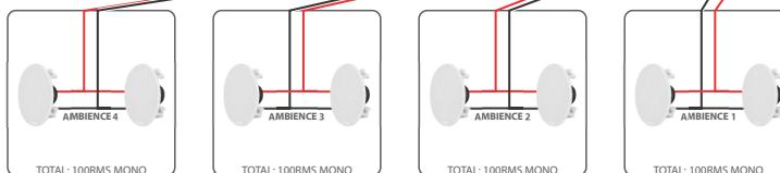
To connect to ceiling speakers, use cables with a minimum gauge of 1.5mm<sup>2</sup> for up to 40 meters. For longer distances, see table on page 02 "Important recommendations". It is necessary to make connections in parallel and series as shown in the example, to match impedance.
