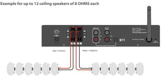
For this kind of connection use cables with a minimum gauge of 1.5 mm<sup>2</sup>(15 AWG) for up to 40 meters (131,2ft). For long distances, consult the table on page 02 in "Important recommendations". It is necessary to make connections in parallel as shown in the example, to match impedance. For other types of projects and installations, consult our technical support.
