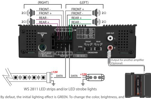
By defaut, the initial lighting effect is GREEN. To change the color, brightness, and effect type, use the remote control in RGB mode (Page 07) or simply press SYNC at rear panel.
