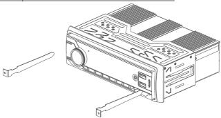
Install the metal bracket into the slot provied for the radio in the vehicle's dashboard and bend the tabs to properly secure the metal bracket in the installation opening.
