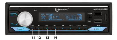
**11 - DISP:** Function to switch between displaying the clock time or displaying playback information.
