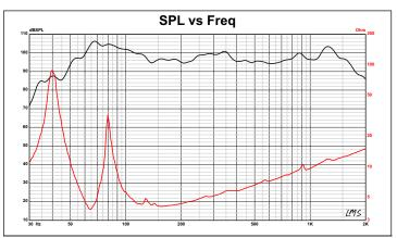
Response curve in a 79,5L box tuned to 63 Hz in an anechoic chamber, 1W / 1M
