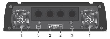
1 - FANS: This amplifier has four internal ventilation fans. For perfect functioning, the amplifier must be installed in a cool and aired place with at least 1"(25mm) space around the heatsink for proper heat spreading.
