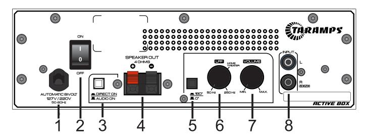
1 - **Power Cable**: Connect the cacle to the electricity network. This product operats with a power supply between 90 and 240 VAC.
