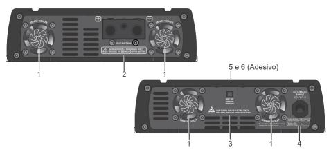
**1 - SMART COOLER:** An intelligent system that controls the operation of fans and ventilation, varying their speed according to temperature and output current. This system ensures a longer lifespan for the fans and provides a quieter ambient as the fans only come into operation only if necessary.
