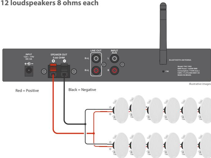
For this kind of connection use cables with a minimum gauge of 1.5 mm<sup>2</sup>(15 AWG) for up to 40 meters (131,2ft). For long distances, consult the table on page 02 in "Important recommendations".
