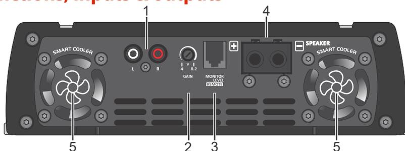
**1 - L/R:** Inputs of signals to be amplified. Connect these signals to RCA outputs of Head Unit, using good quality shielded cables to avoid noise influence.
