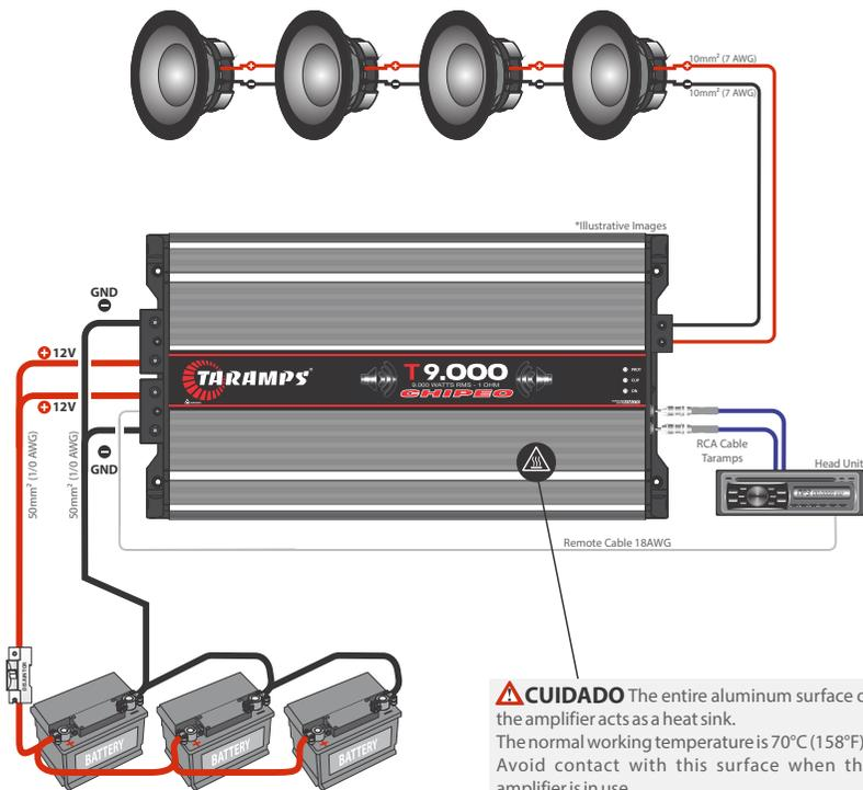
**CAUIDADO** The entire aluminum surface of the amplifier acts as a heat sink. The normal working temperature is 70°C (158°F). Avoid contact with this surface when the amplifier is in use.
