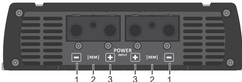
**1 - NEGATIVE POWER SUPPLY TERMINAL:** A 1/0 AWG (50mm<sup>2</sup>) cable as short as possible must be used, connected to the negative battery pole.
