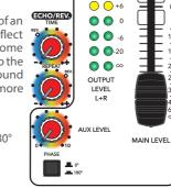
**PHASE** Inverts the signal phase of the AUX OUT channel by 180°
