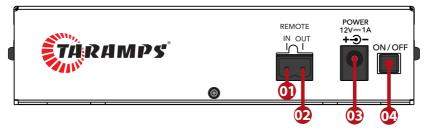
The **T 0302 FX MULTICOLOR** was designed to be used in car audio systems with a 12V battery, but it can also be used with an external 12V plug adapter with a current of at least 2A, which must be purchased separately (in this case, the consumer should pay attention to the adapter plug that should be standard P4-2mm). It has an ON/OFF button that eliminates the REMOTE IN connections.
