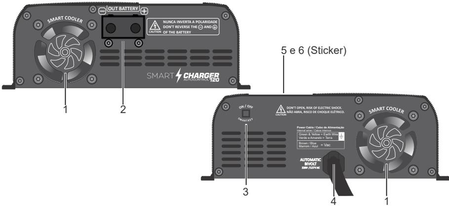
**1 - SMART COOLER:** An intelligent system that controls the operation of coolers and ventilation, varying their speed according to temperature and output current. This system ensures a longer lifespan for the coolers and provides a quieter ambient as the coolers only come into operation only if necessary.
