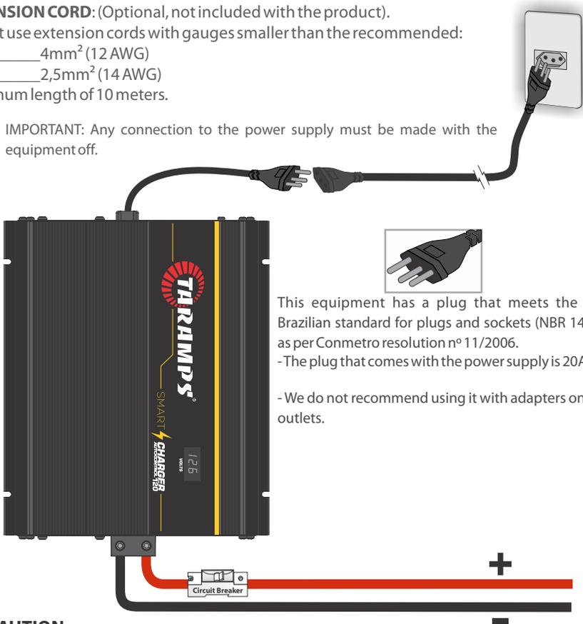
This equipment has a plug that meets the new Brazilian standard for plugs and sockets (NBR 14136) as per Conmetro resolution nº 11/2006.
