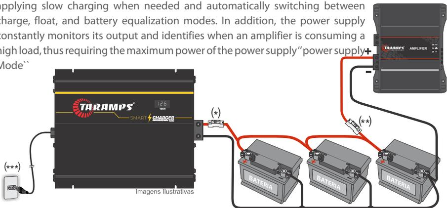
(\*) Use circuit breaker as indicated in the manual for each power supply.
