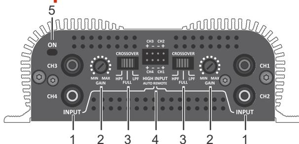
**1 - INPUT:** Inputs of signals to be amplified. Connect these signals to RCA outputs of Head Unit, using good quality shielded cables to avoid noise interference.
