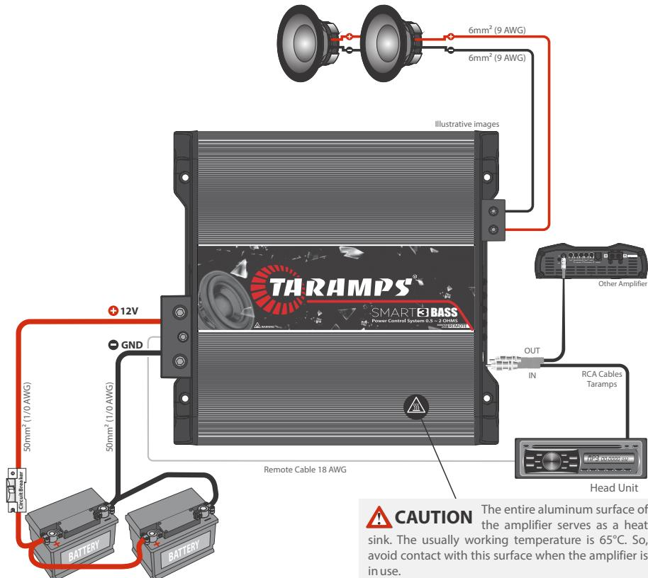
Examples of connections in the power supply input.
