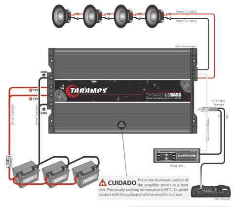
Examples of connections in the power supply input. Note: Required battery bank capacity: At least 230Ah
