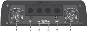
1 - SMART COOLER: This amplifier has two internal ventilation fans. For perfect functioning, the amplifier must be installed in a cool and aired place with at least 1"(25mm) space around the heatsink for proper heat spreading. The usually working temperature of amplifier is 65°C.
