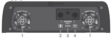
1 - SMART COOLER: This amplifier has two internal ventilation fans. For perfect functioning, the amplifier must be installed in a cool and aired place with at least 1" (25mm) space around the heatsink for proper heat spreading. The usually working temperature of amplifier is 65°C.
