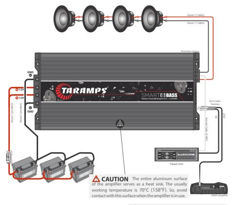
Examples of connections in the power supply input. Note: Required battery bank capacity: At least 360A
