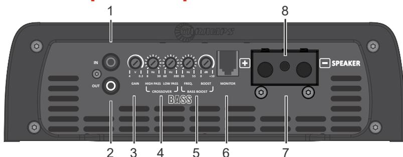
**1 - IN:** Input of signal to be amplified. Connect the to the RCA output of the Head Unit using good shielded cable to avoid noise interference.
