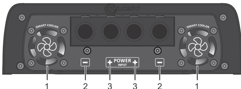
**1 - SMART COOLER:** This amplifier has two internal ventilation coolers, which cannot be obstructed. Controlled by an intelligent system (Smart Cooler), it only operates at full speed when needed, ensuring longer cooler life and a quieter operation of your amplifier. For a perfect operation, the amplifier must be installed in a dry and airy place. We recommend not embedding it, in order to ensure adequate ventilation.
