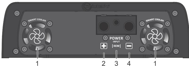
**1 - SMART COOLER:** This amplifier has two internal ventilation coolers, which cannot be obstructed. Controlled by an intelligent system (Smart Cooler), it only operates at full speed when needed, ensuring longer cooler life and a quieter operation of your amplifier. For a perfect operation, the amplifier must be installed in a dry and airy place. We recommend not embedding it, in order to ensure adequate ventilation.
