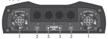
**1 - SMART COOLER:** This amplifier has four internal ventilation fans. For perfect functioning, the amplifier must be installed in a cool and aired place with at least 1''(25mm) space around the heatsink for proper heat spreading. The usually working temperature of amplifier is  $70^{\circ}$ C ( $158^{\circ}$ F).
