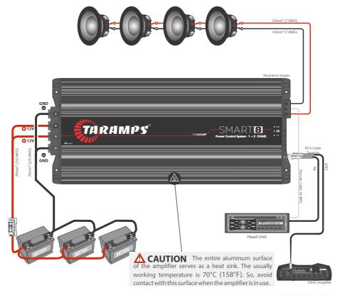
Examples of connections in the power supply input. Note: Required battery bank capacity: At least 400Ah
