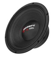
The ML 500S model was designed to faithfully reproduce bass and midrange, responding from 55Hz to 3,200Hz. Its ventilated housing provides an efficient heat exchange that preserves the coil, rated at 250 watts RMS. The ML 500S can be used in a variety of sound systems.
