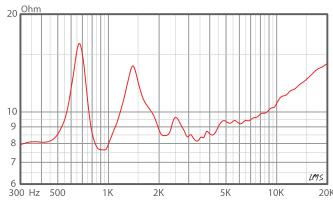
Impedance curve obtained without horn
