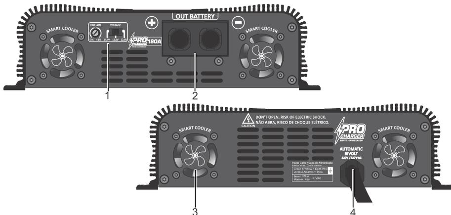
1 - VOLTAGE / FINE ADJ: Select the output voltage: 12.6V, 13.8V or 14.4V. The output voltage can be set to  $\pm 3\%$  by the FINE ADJ feature, observing the voltage in the voltmeter.
