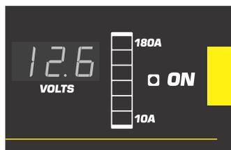
LED ON: The ON (led indicator) keep on while the power supply is connected at AC POWER.
