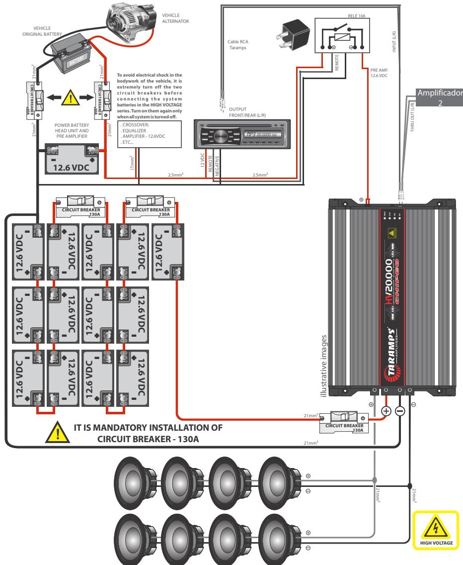
\* Gauge for the output cable is 21mm<sup>2</sup>, calculated a maximum length of 2m.
