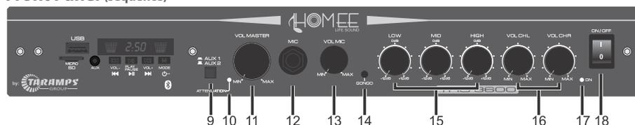
**9 -AUX1 / OPTICAL or AUX 2 KEY:** Button pressed: Selects AUX1 and Optical inputs.
