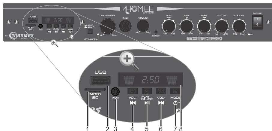
**1 - MICRO SD:** Micro SD memory card input.
