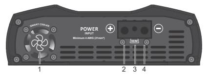
1 - FAN: This amplifier has one internal ventilation fan. For perfect functioning, the amplifier must be installed in a cool and aired place with at least 1" (25mm) space around the heatsink for proper heat spreading. The usually working temperature of amplifier is 65°C.
