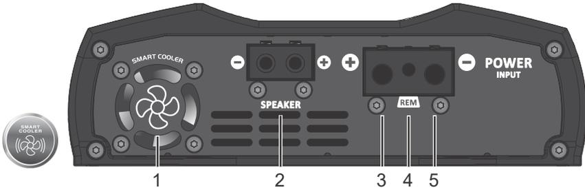
**1 - FAN:** This amplifier has one internal ventilation fan. For perfect functioning, the amplifier must be installed in a cool and aired place with at least 1" (25mm) space around the heatsink for proper heat spreading. The usually working temperature of amplifier is 65°C.
