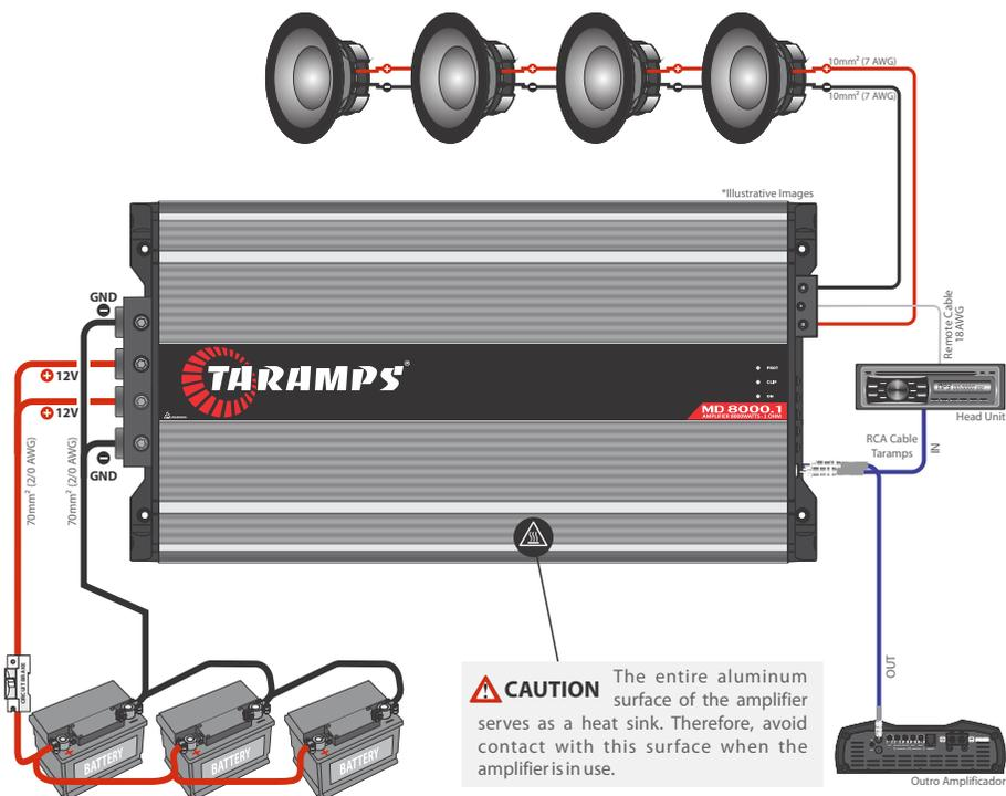
**CAUTION** The entire aluminum surface of the amplifier serves as a heat sink. Therefore, avoid contact with this surface when the amplifier is in use.
