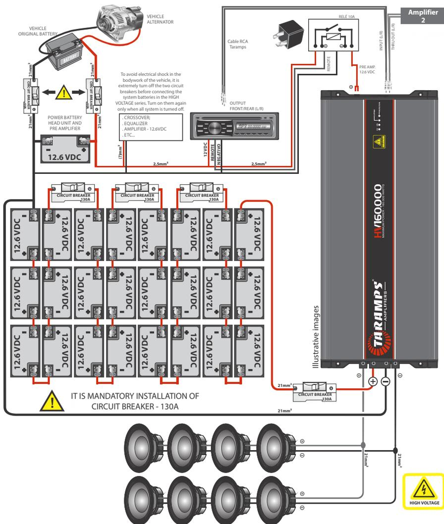
\* Gauge for the output cable is 21mm<sup>2</sup>, calculated a maximum length of 2m.
