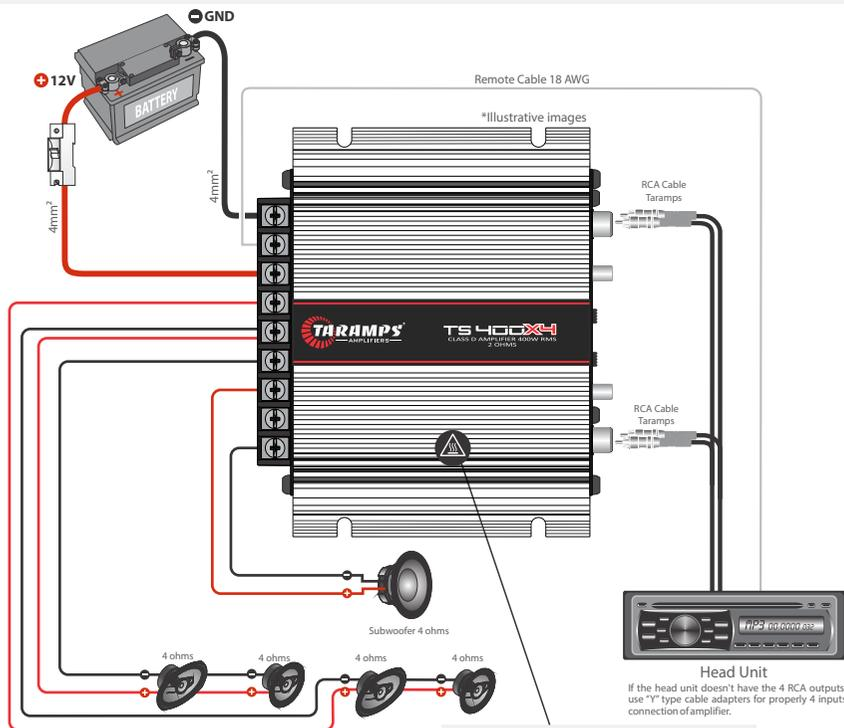
Connection example in the output: Stereo + Bridged
