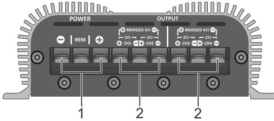
**1 - POWER (Power Supply Connector):** The connector terminal (+) must be connected to the battery's positive pole with a 4mm<sup>2</sup> (minimum) wire gauge. The connector terminal (-) must be properly connect to the battery's negative pole with a same wire gauge. The remote terminal must be connected to the Head Unit REMOTE output with a 0.75mm<sup>2</sup> wire.
