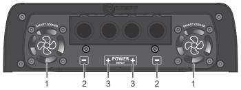
1 - SMART COOLER: This amplifier has six internal ventilation fans. For perfect functioning, the amplifier must be installed in a cool and aired place with at least 1" (25mm) space around the heatsink for proper heat spreading. The usual working temperature of this amplifier is 70°C (158°F).
