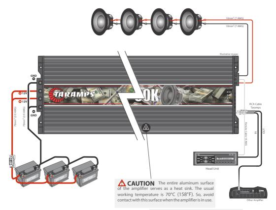
Examples of connections in the power supply input. Note: Required battery bank capacity: At least 1150Ah
