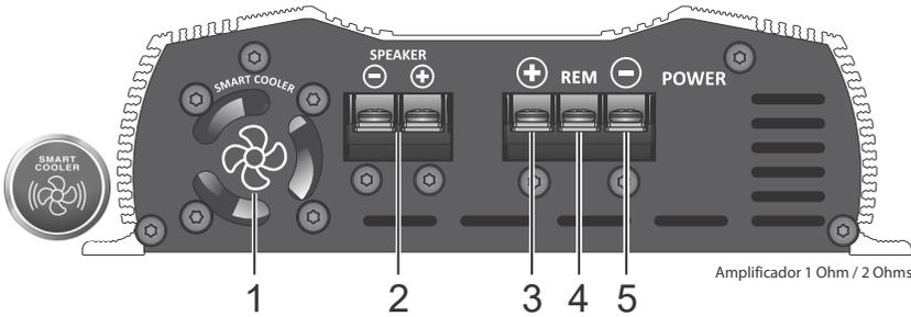
**1 - FAN:** The BASS 800, has one internal fan, and cannot be blocked. This fan is controlled by an intelligent system (**Smart Cooler**). The fan only runs at maximum speed after the product reach a certain temperature level. This function ensures long fan life and silent operation of your amplifier.
