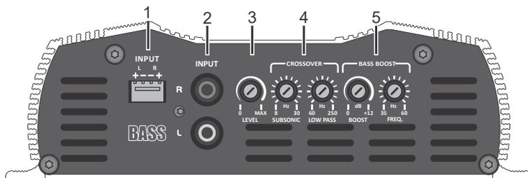
**1 - INPUT FOR SIGNALS L / R (HIGH LEVEL):** Signal connectors to be amplified. Connect them to the hi-level output connections (WIRES) from CD / DVD player.
